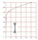
In case the stress-strain-curve is determined by a tensile test according DIN standard, a text file or an Excel table with the value pairs of stress and strain can be imported. To check the imported values, the curve is displayed graphically.
