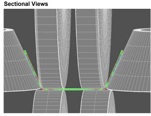
Sectional views of the sheet within the rolls, at any machine position, or after leaving the machine are created by key-press. The rolls can be inserted (as 2D cross section or as 3D solids alternatively) in order to check the position of the sheet within the roll tools. Inserting the designed flower pattern enables target/actual comparison.
