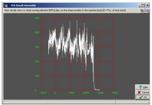
The **PROFIL** postprocessor creates graphs that show the transversal and longitudinal stress, the strain, and the sheet thickness reduction as a function of the sheet position in the machine. These graphs are tailored to the special needs of roll form designers and help to evaluate the FEA result.
