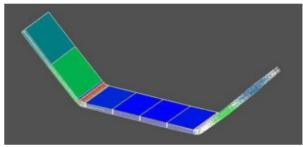
Running of a flat sheet into a stand with 45 degree rolls was simulated. Without clearance angles considerable strain is shown in the legs (green: medium strain).
