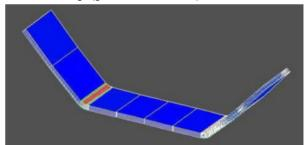
With clearance angles the legs are not strained (blue color). The red color shows high plastic strain in the bending zones, which is necessary that the profile does not spring back after leaving the machine.
